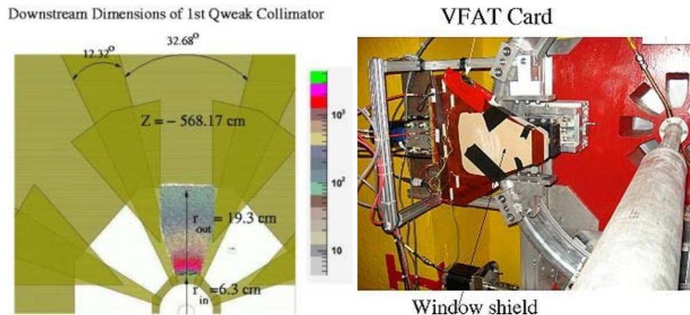
Figure 1. Left: A view of the simulated electron profile overlaid on top of the final collimator design. Right: A picture of the detector installed in Hall C for testing before the commissioning run.
