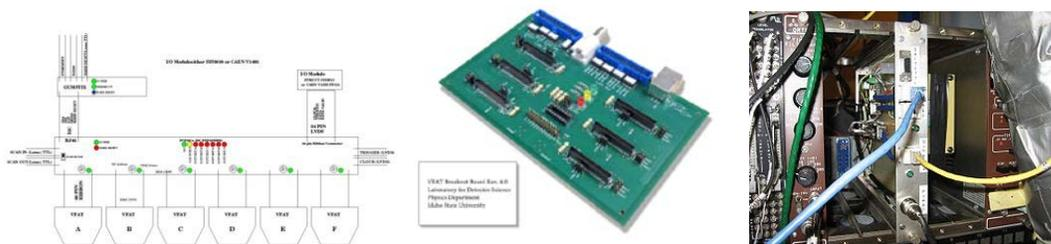
Figure 3. The VFAT readout system. Left: a block diagram of the control system. Middle: A breakout board designed at ISU to direct control and data signals. Right: A NIM bin module built at ISU to power the readout electronics and house the slow controls computer.
