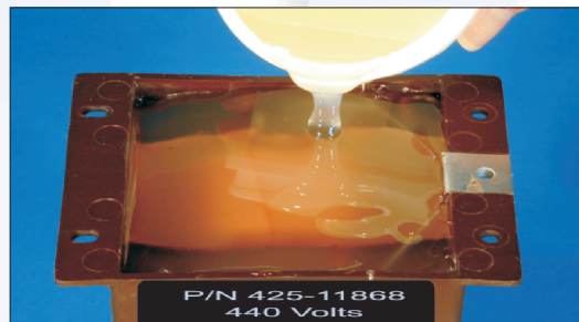
4461 Potting a Transformer for High Temp. Use
