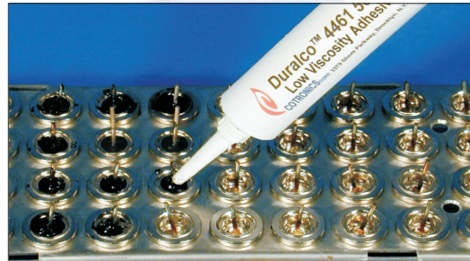
4461 Penetrates and Encapsulates A Semi-Conductor Device
