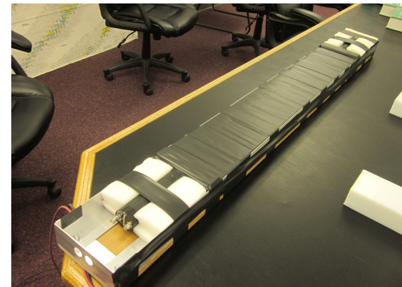
(left) 30" x 6" x 1.5" scintillators. Light guides and PMT on each end. Wrapped in reflective material. Position information to within ± 10 cm obtained by timing delay between PMT's mounted at the two ends.
