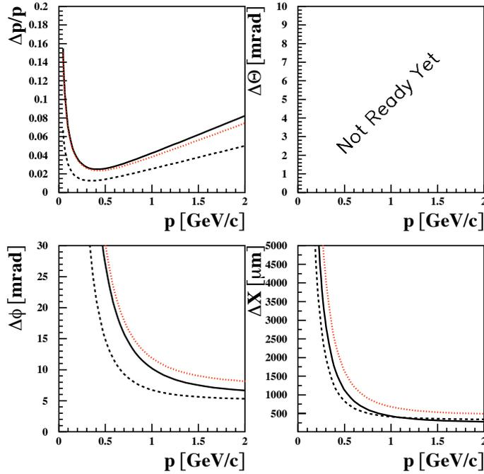
Figure 5: Resolution plotted versus particle momentum for 90 deg tracks. Subfigures a, b, c and d show the momentum, theta, phi and vertex resolutions, respectively. Three options are shown: solid- 3 SVT planes; dashed- 16 DC-stereo planes; dotted - 8 DC-cathode pad planes
