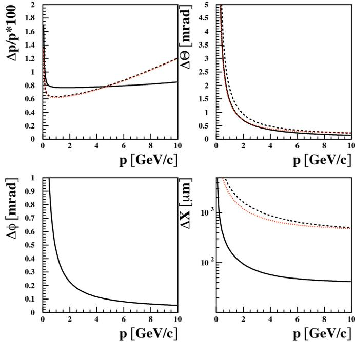
Figure 4: Resolution plotted versus particle momentum for 30 deg. tracks. Sub-figures a, b, c and d show the momentum, theta, phi and vertex resolutions, respectively. Three options are shown: solid- 3 SVT planes + CC + 3 DC planes; dashed- CC + 3 DC planes; dotted - 3 DC planes
