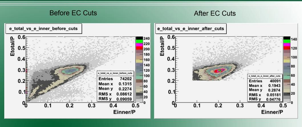
Cuts on the energy deposited in the electromagnetic calorimeter (ECtotal>0.2\*p and ECinner>0.06\*p)
