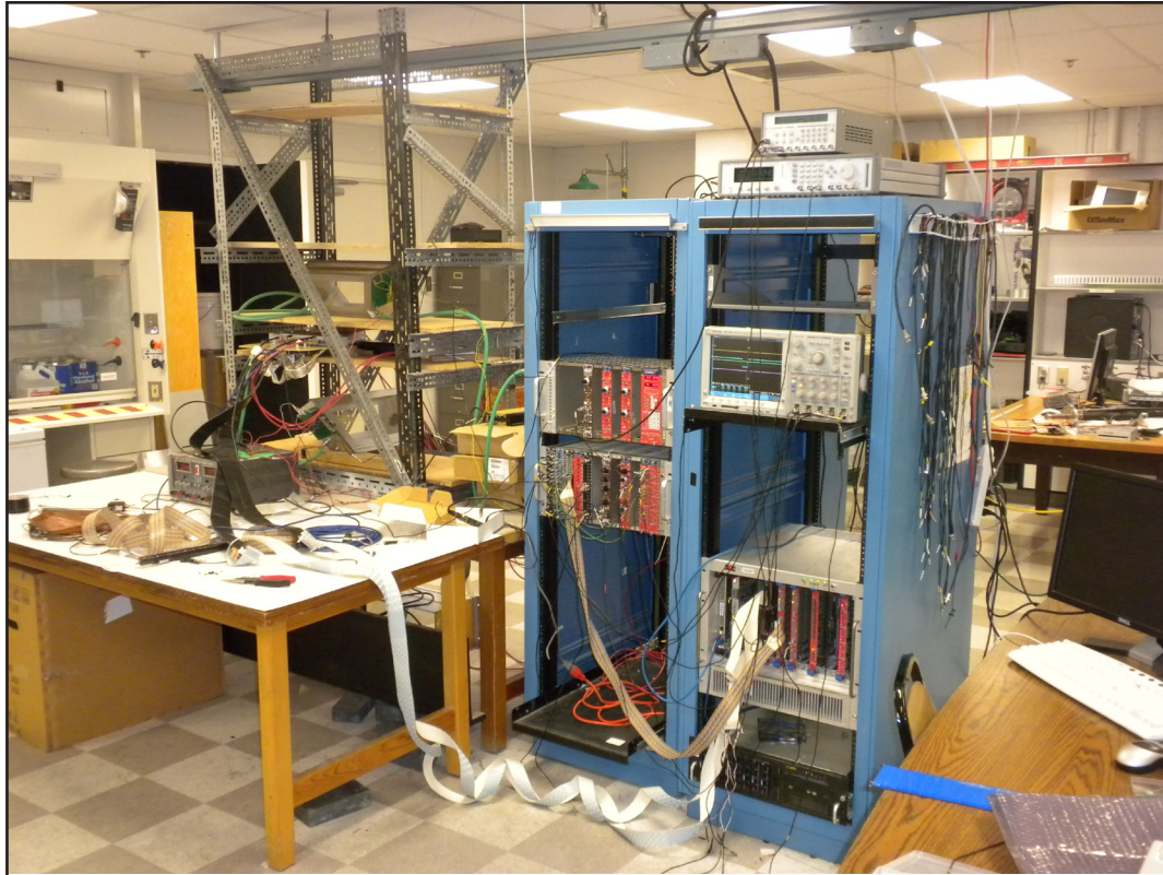
Figure 1-4: A typical setup of the Region 1 detector including VME crate
