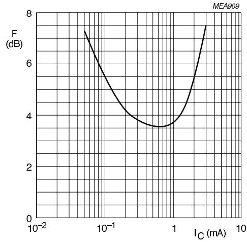
$V_{CE} = 1$  V;  $Z_S = \text{opt.}$ ;  $f = 500$  MHz;  $T_{amb} = 25$  °C.
