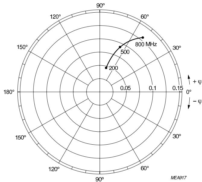
$I_C = 1 \text{ mA}; V_{CE} = 1 \text{ V}; T_{amb} = 25^\circ\text{C}.$ Fig.8 Common emitter reverse transmission coefficient ( $S_{12}$ ).
