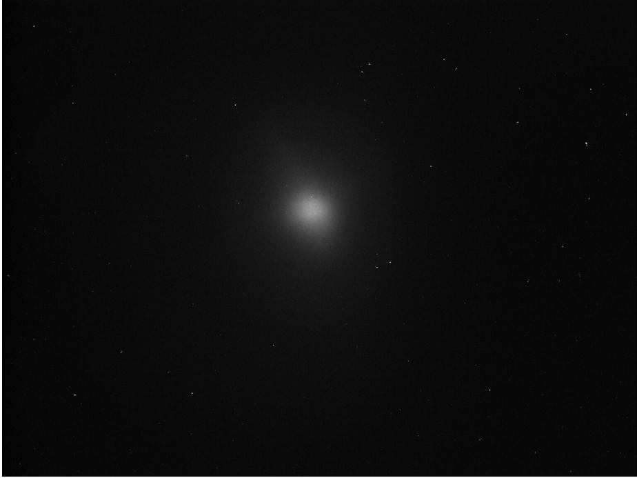
Figure 3.2: The 15 MeV electron beam observed using the OTR screen when dipole coil current was at 0. The macro pulse was 200 ns and the electron peak current was 40 mA .
