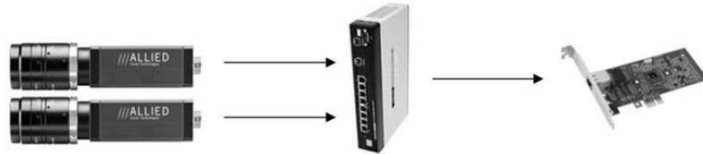
Figure 24: Multi camera network configuration using a switch and single Ethernet port
