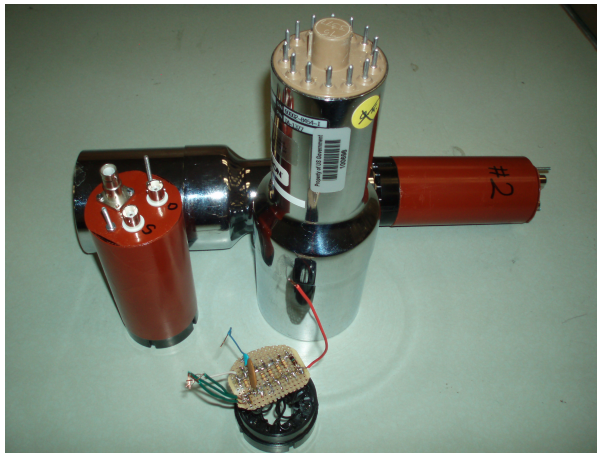
Figure 4: The NaI detector and base built.
