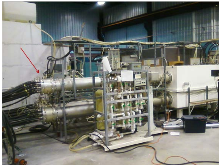
Fig.1 ISIS induction cell driver. The future position of the impedance transformer is indicated by the red arrow.
