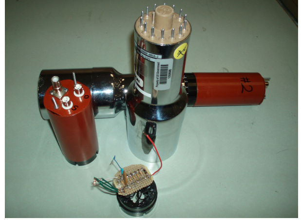
Figure 4: The NaI detector and base built.
