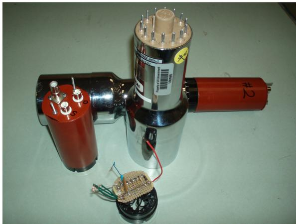
Figure 4: The NaI detector and base built.
