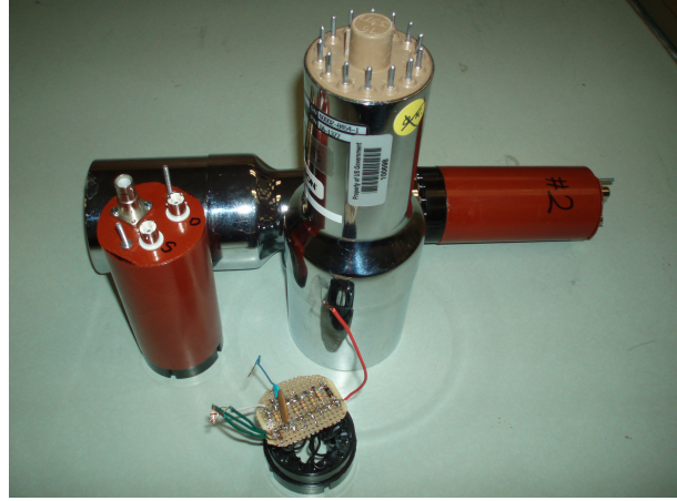
Figure 4: The NaI detector and base built.
