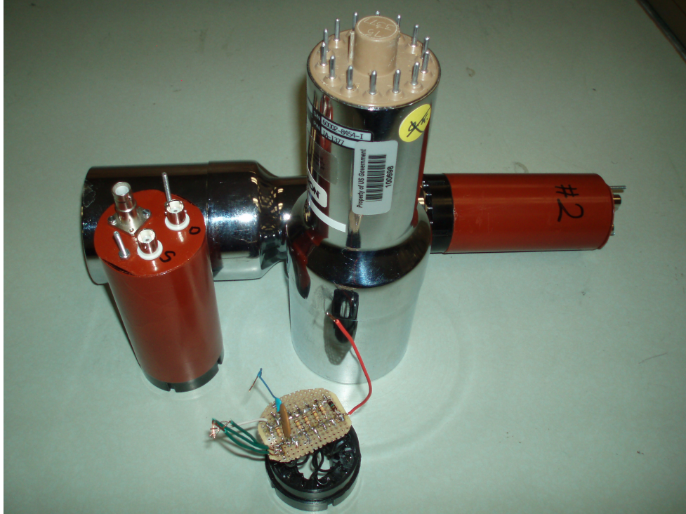
Figure 2.7: The NaI crystals and new bases.
