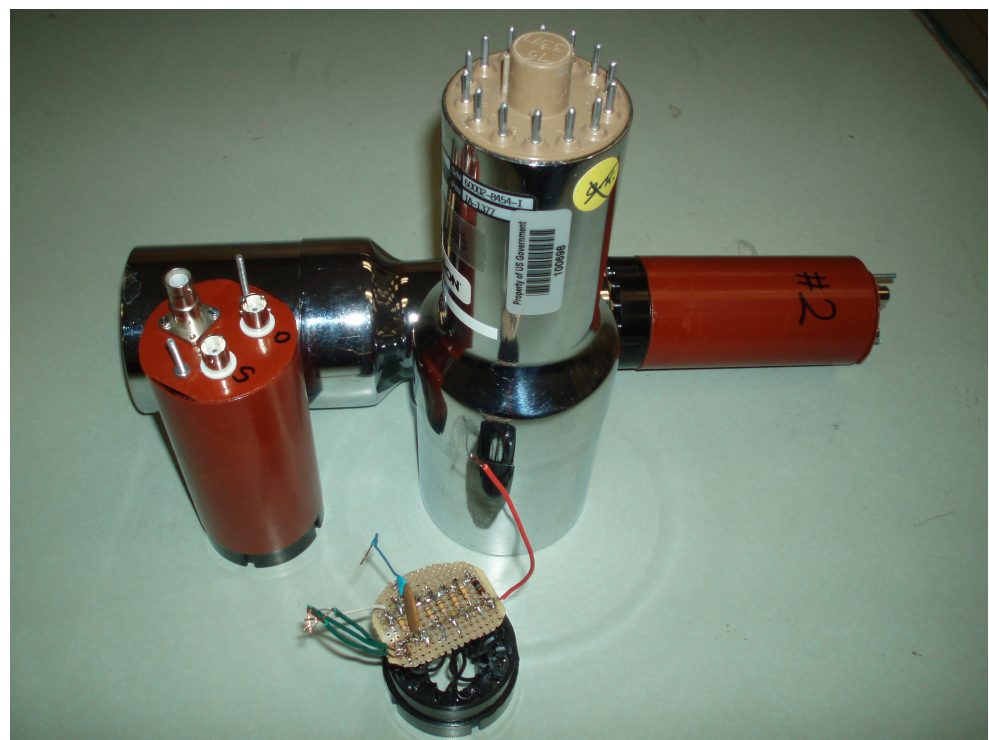
Figure 2.7: NaI crystals and new bases.
