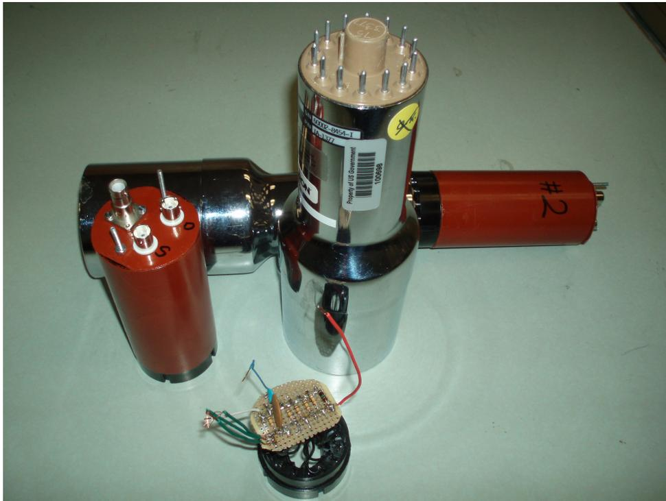
Figure 3.11: NaI crystals and new bases.
