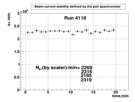
The pair converter thickness should be adjusted such that the number of positrons produced per minute is less than f(Hz)\*60(s) for a given electron current and given thickness of the bremsstrahlung converter. In this case it is possible to see the response of the pair spectrometer to the change of the photon flux.
