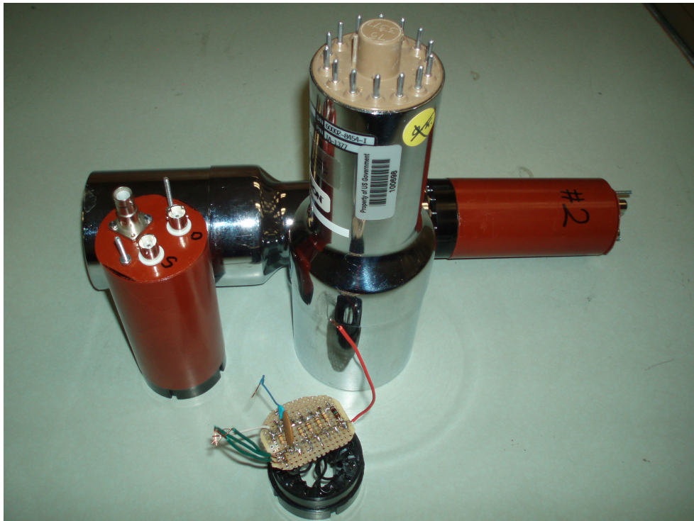
Figure 2.4: Sodium Iodide (NaI) detector and parts.
