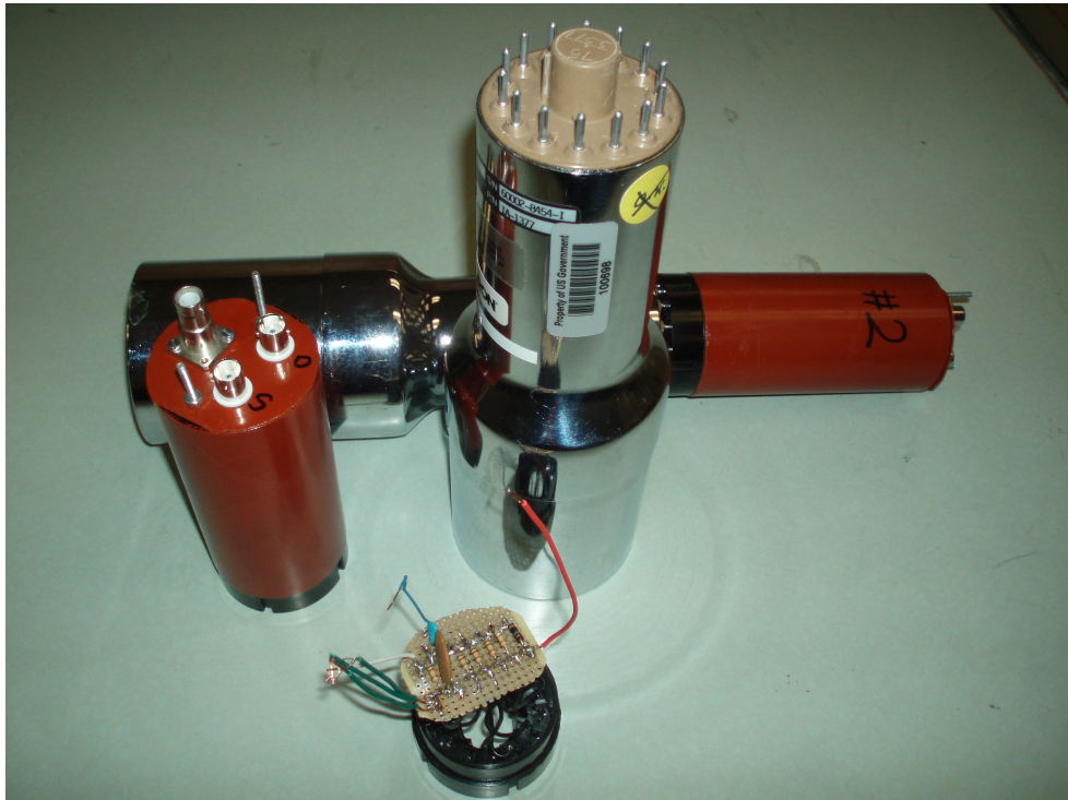
Figure 2.4: Sodium Iodide (NaI) detector and parts.
