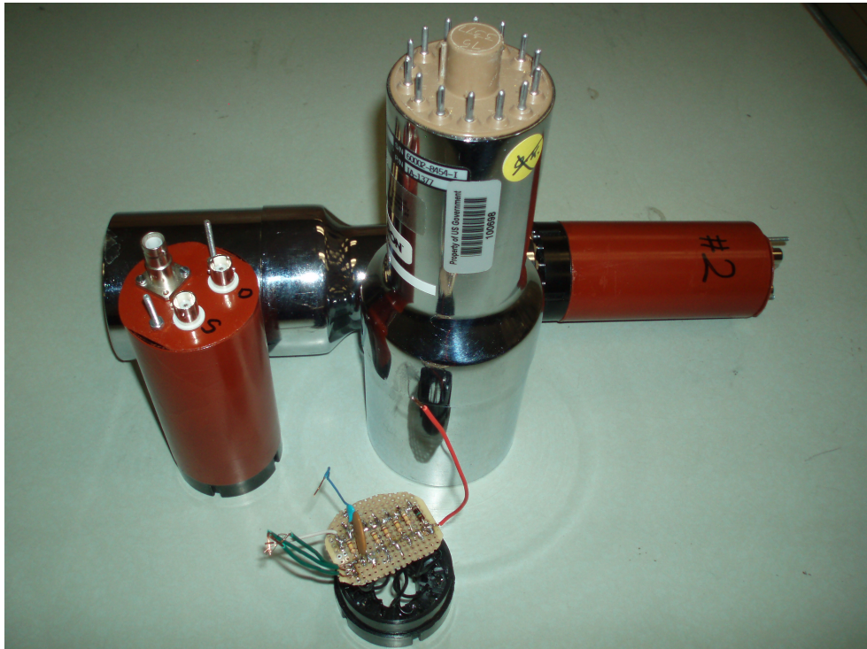
Figure 2.4: Sodium Iodide (NaI) detector and parts.
