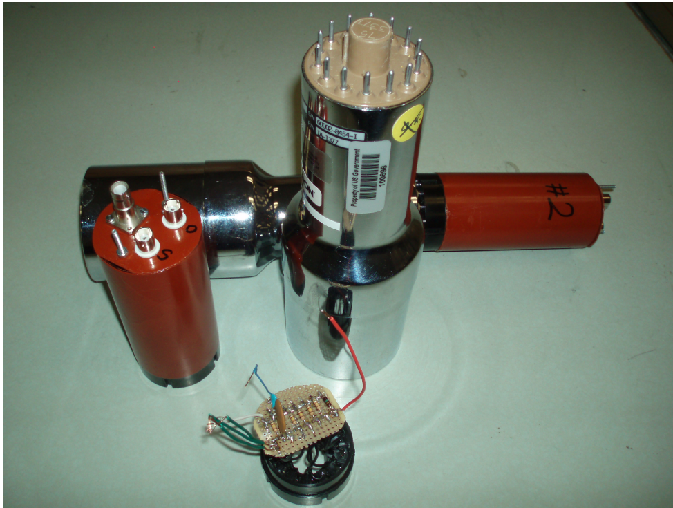
Figure 2.4: Sodium Iodine (NaI) detector and parts.
