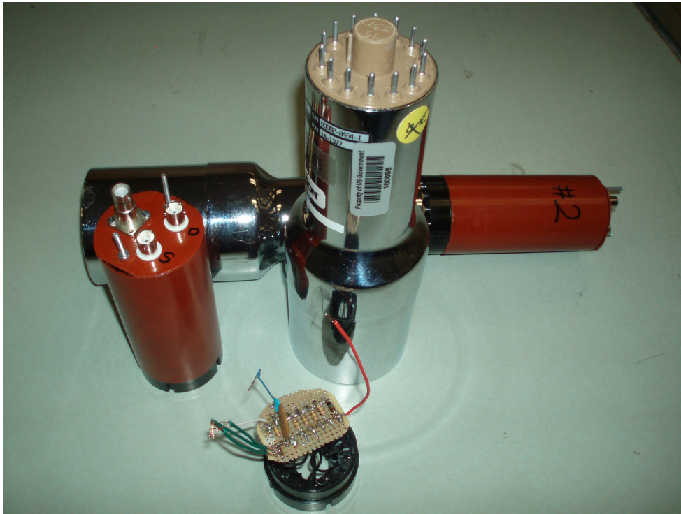
Figure 2.4: Sodium Iodine (NaI) detector and parts.
