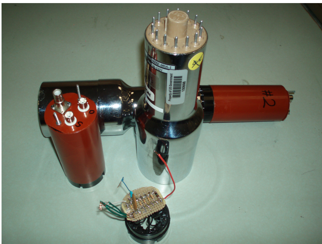
Figure 2.4: Sodium Iodide (NaI) detector and parts.
