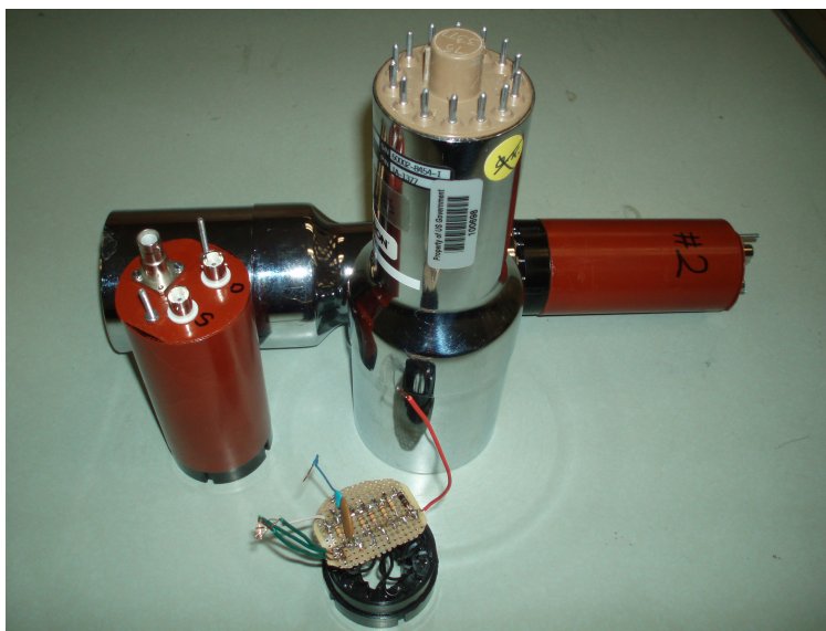
Figure 2.4: Sodium Iodide (NaI) detector and parts.
