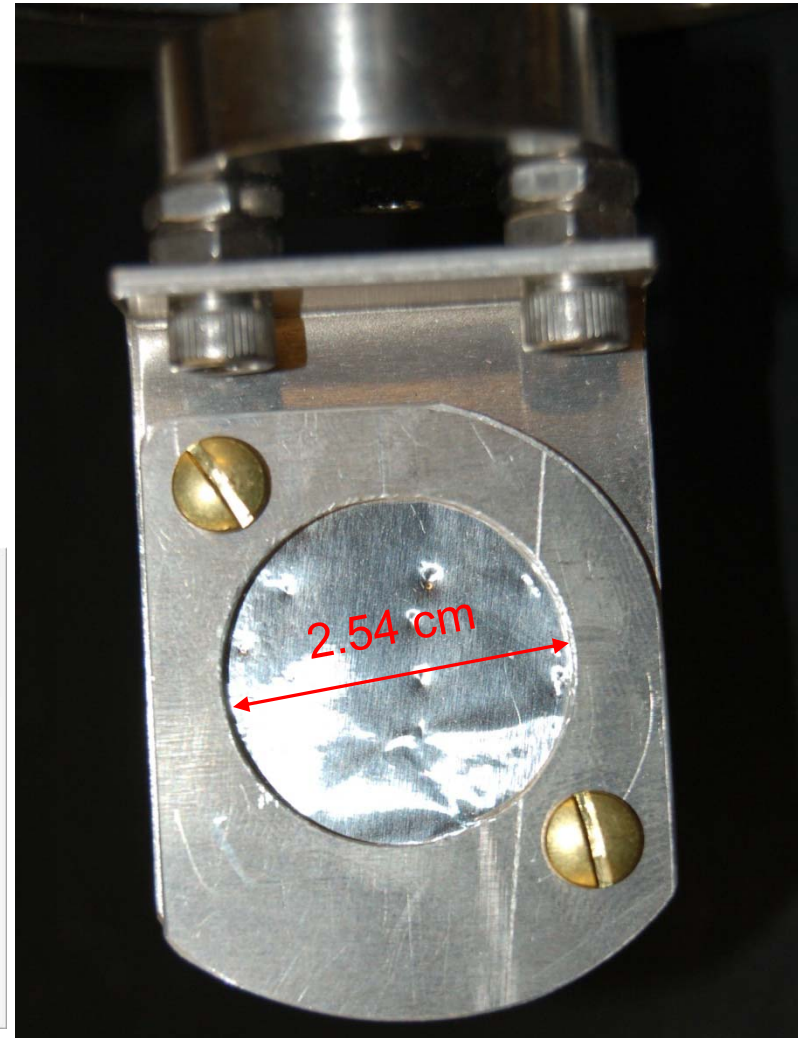
Figure 46: Radiator mounting bracket used to attach the radiator to the ladder to provide an in, or out, or the beam ability. Measurements reveal the inner diameter of the holder may be interfering with the electron beam.
