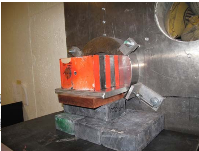
Figure 13: Off-axis collimation used to transport linearly polarized bremsstrahlung into the experimental cell for experimentation.
