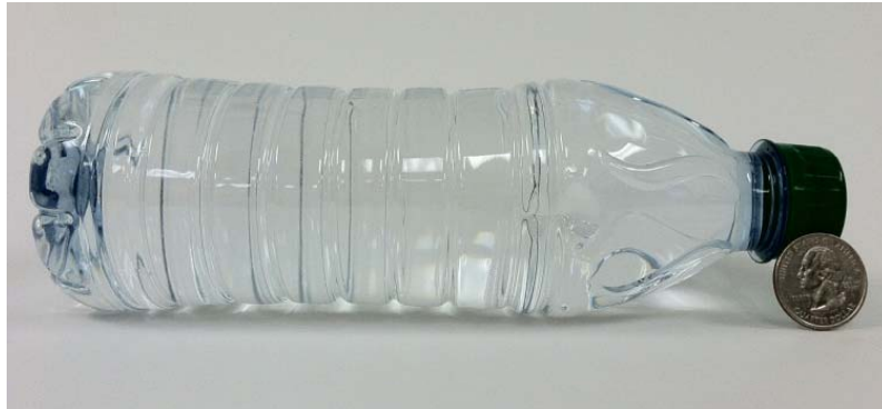
Figure 33: D 2 O target used to measure the polarization of the off-axis bremsstrahlung beam.
