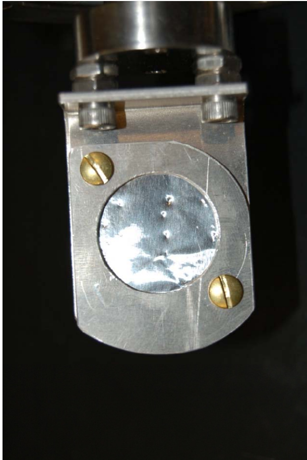
Figure 9: 1/2 mil Al radiator attached to a ladder.
