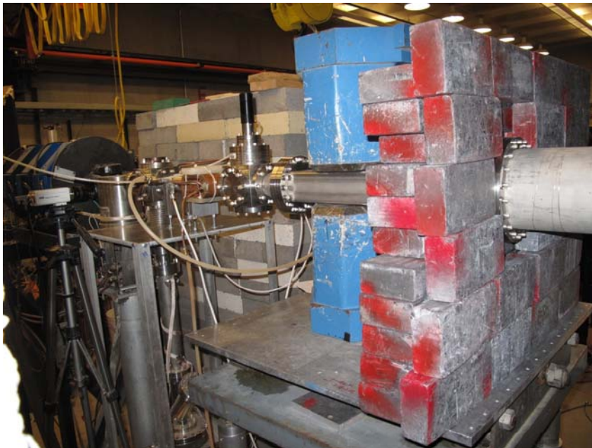
Figure 23: Charged particles are swept from the beam line using a 3kG x 20cm permanent magnet, and dumped into a graphite and lead beam dump.
