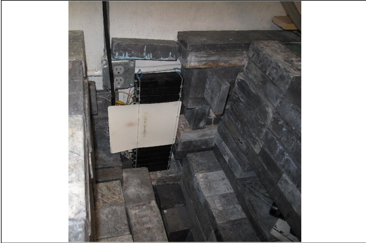
Figure 7: Segmented Faraday cup composed of 16 stacked aluminum bricks just upstream of shielding wall on accelerator side, view screen attached to upstream side of that with camera placed next to the kicker magnet.
