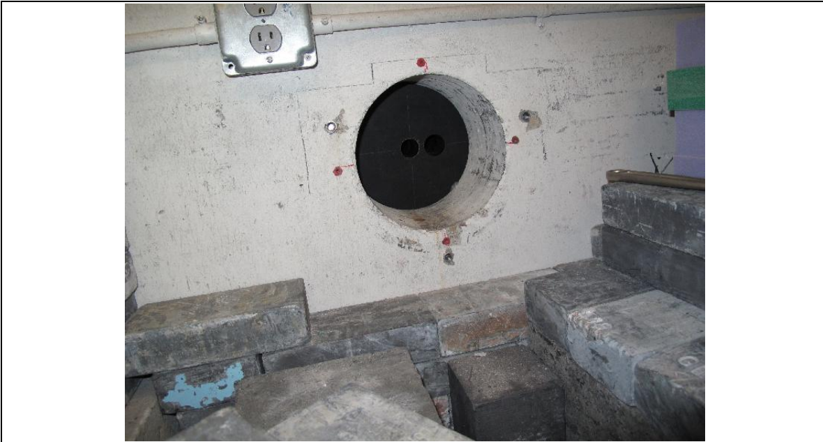
Figure 3: A 12-inch thick off axis collimator at m/E beam right, \Delta\theta = m/(2E) .
