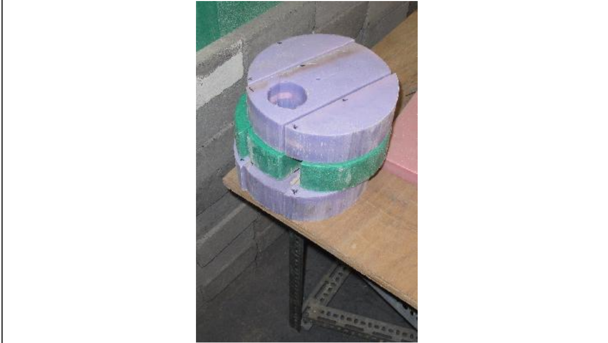
Figure 9: 6-inch thick neutron shielding with off axis hole placed downstream of the 12-inch thick off-axis collimator.
