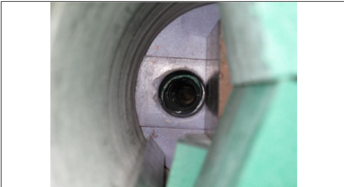
Figure 10: An 8-inch copper brick was used to cover the central hole of the 12-inch thick off-axis collimator. The rest of the space in the hole of the concrete wall was filled with borated polyethylene without covering the off axis collimator hole.
