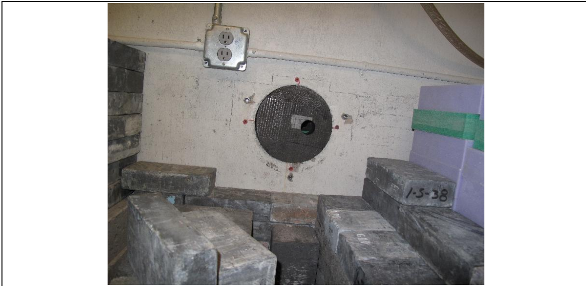
Figure 6: 2-inch thick graphite shielding with off axis hole downstream of the Faraday cup.
