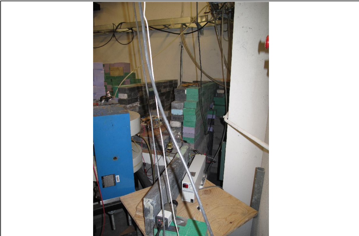
Figure 2: The kicker magnet power supply and monitoring camera placed behind lead shielding.
