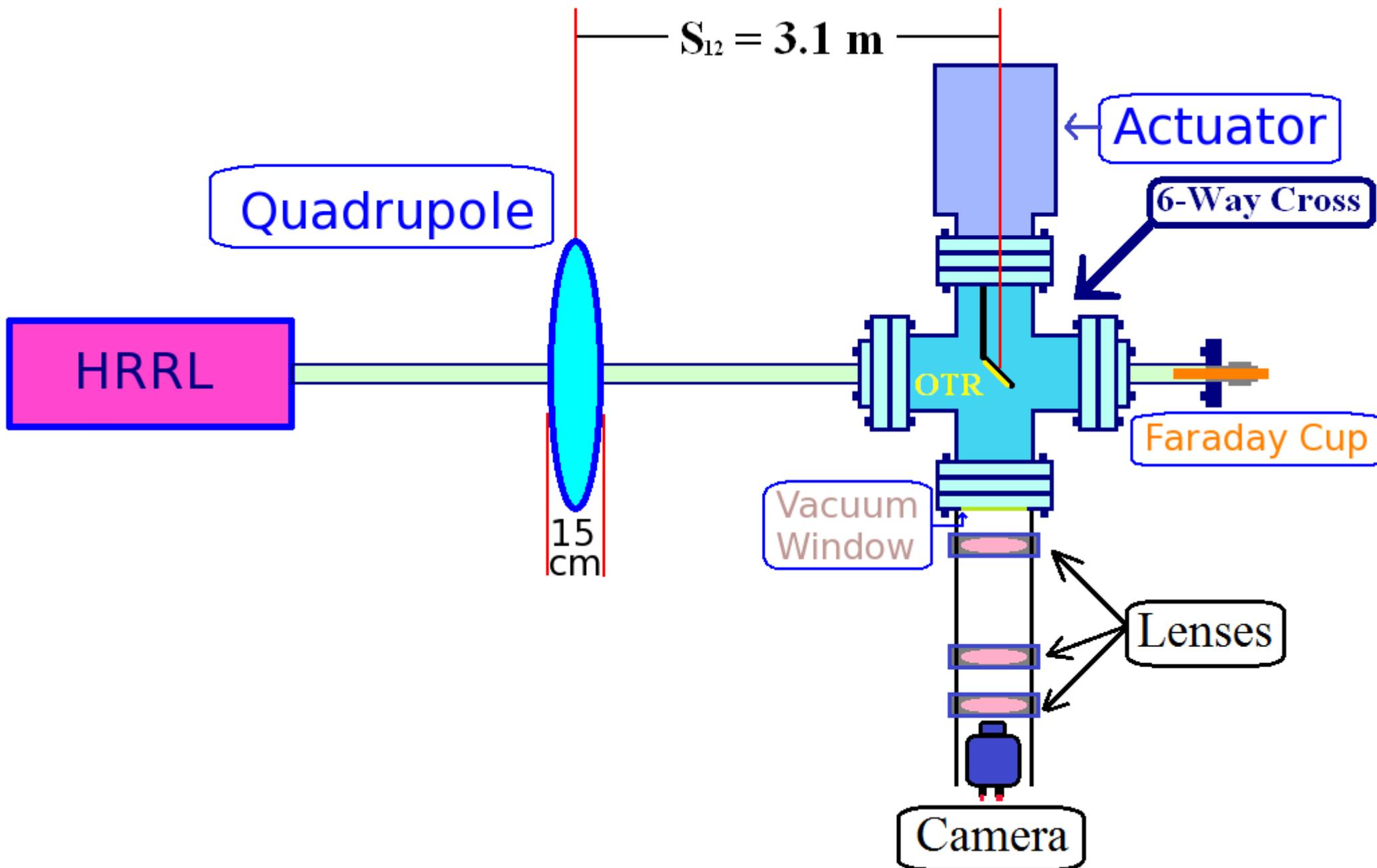
**Optical Transition Radiation (OTR):** Transition radiation is emitted when a charge moving at a constant velocity cross a boundary between two materials (Al, Si) with different dielectric constant.
