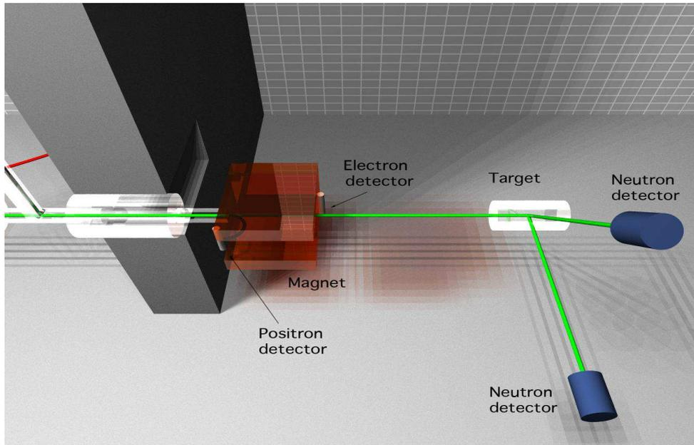
Figure 5: A schematic of the proposed pair spectrometer luminosity monitor (red). Photons entering the experimental hall impinge upon a thin ( $10^{-3}$  radiation length) pair converter. Electrons and positrons are momentum analyzed in a magnet, and detected in plastic scintillator detectors. Target (white) and neutron detectors (blue) are also shown.
