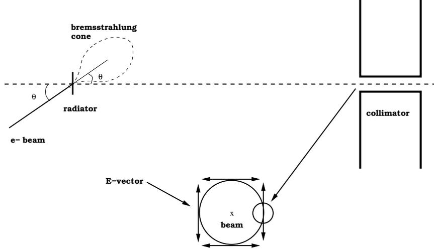
Figure 3: Production of linearly polarized photons by the off axis bremsstrahlung technique. An electron beam strikes a thin ( $\sim 10^{-3}$  radiation length) radiator, and a downstream collimator passes photons whose trajectories lie off axis from the incident electron beam. The optimal angle,  $\theta$ , was chose to be  $2^\circ$  for the proposed experiment to optimize photon intensity and polarization.
