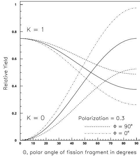
Figure 1:  $\theta$  distribution of fission fragments with photon beam polarization of 30% for  $K = 0, 1$  and  $\phi = 0, 90^\circ$ .  $K$  is the quantum number denoting the projection of the spin of the transition state on the symmetry axis of the deformed fissioning nucleus. Solid lines are for unpolarized photons.
