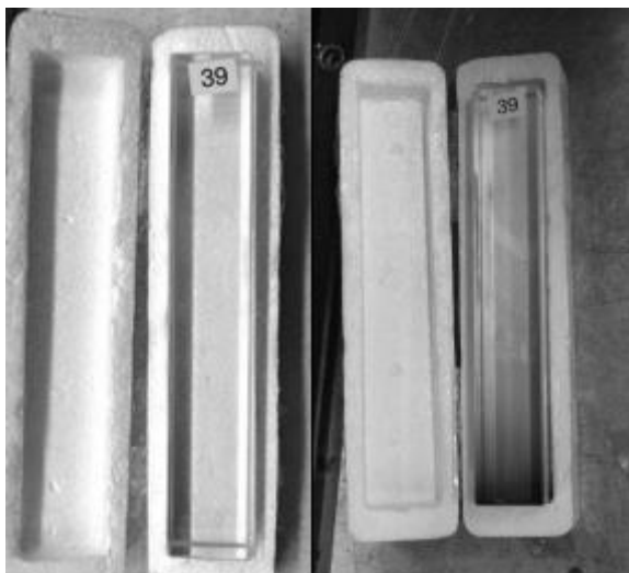
FIGURE 1. Photographs of block 39 before (left) and after (right) irradiation. The beam was incident on the bottom (small) face.
