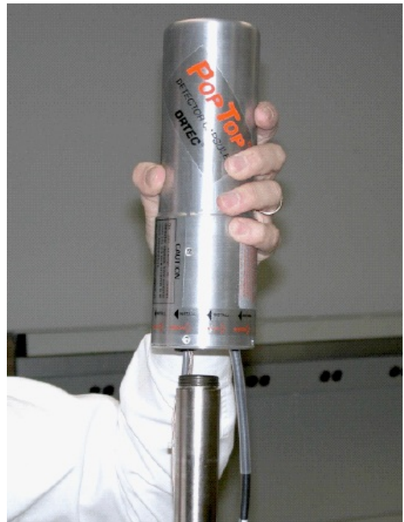
Fig. 2. Coupling of PopTop Capsule to X-Cooler.
