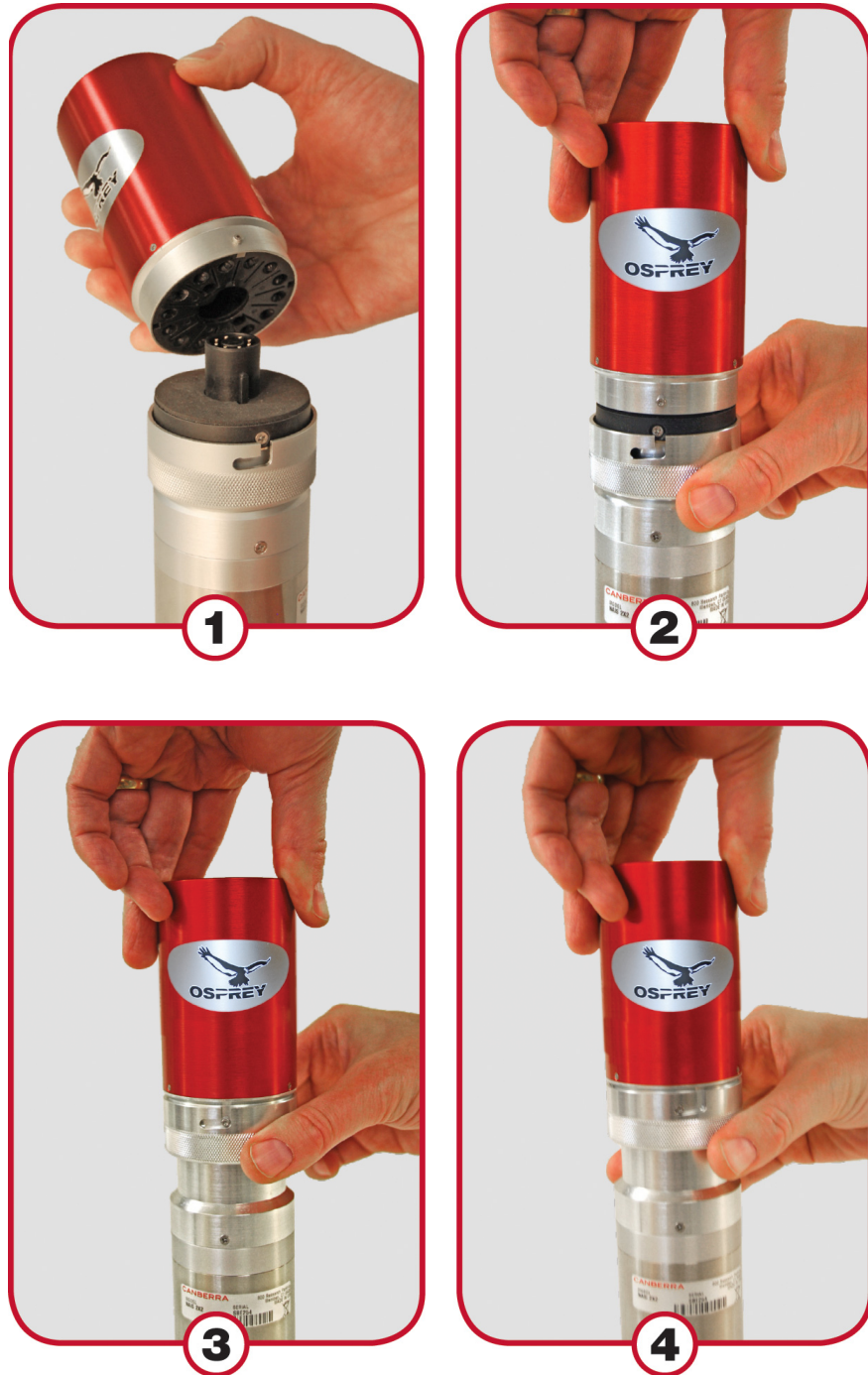
Figure 27 Connecting the Osprey to an 8-Pin Stabilized Probe
