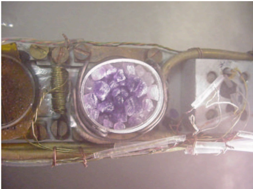
Fig. 2.5: EG1b target material after the radiation damage.
