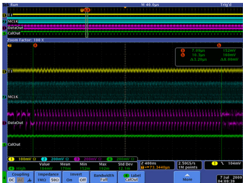
Figure 4-21: CalPulse applied with all odd channels turned on
