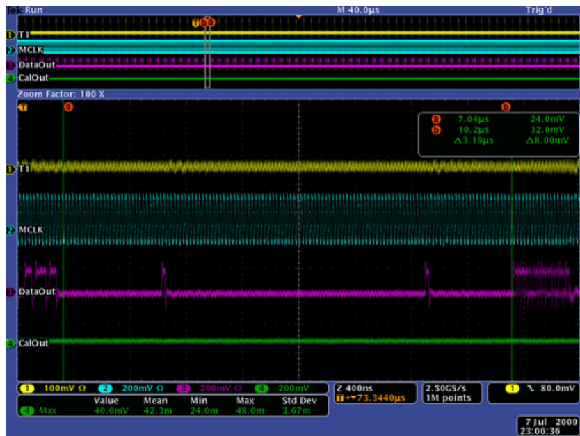
Figure 4-22: CalPulse applied with all odd channels turned on
