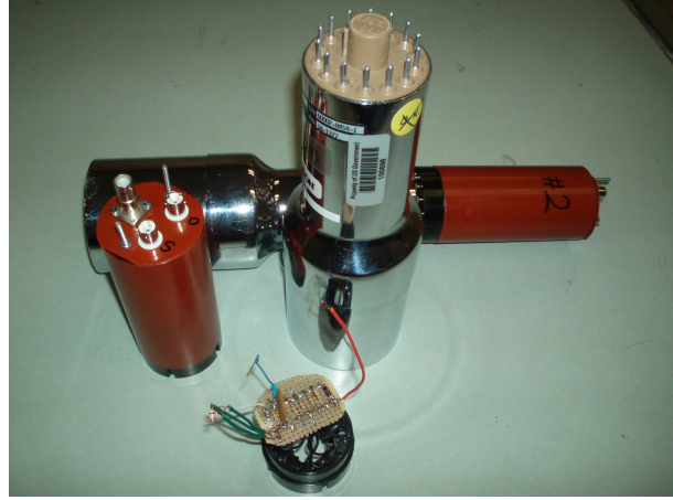
Figure 4: The NaI detector and base built.
