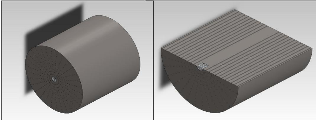
Figure 7. A schematic drawing of the thermal neutron source. A high Z material cylinder will be surrounded by a thick layer of moderating material (for example D<sub>2</sub>O), which will have cavities for samples.
