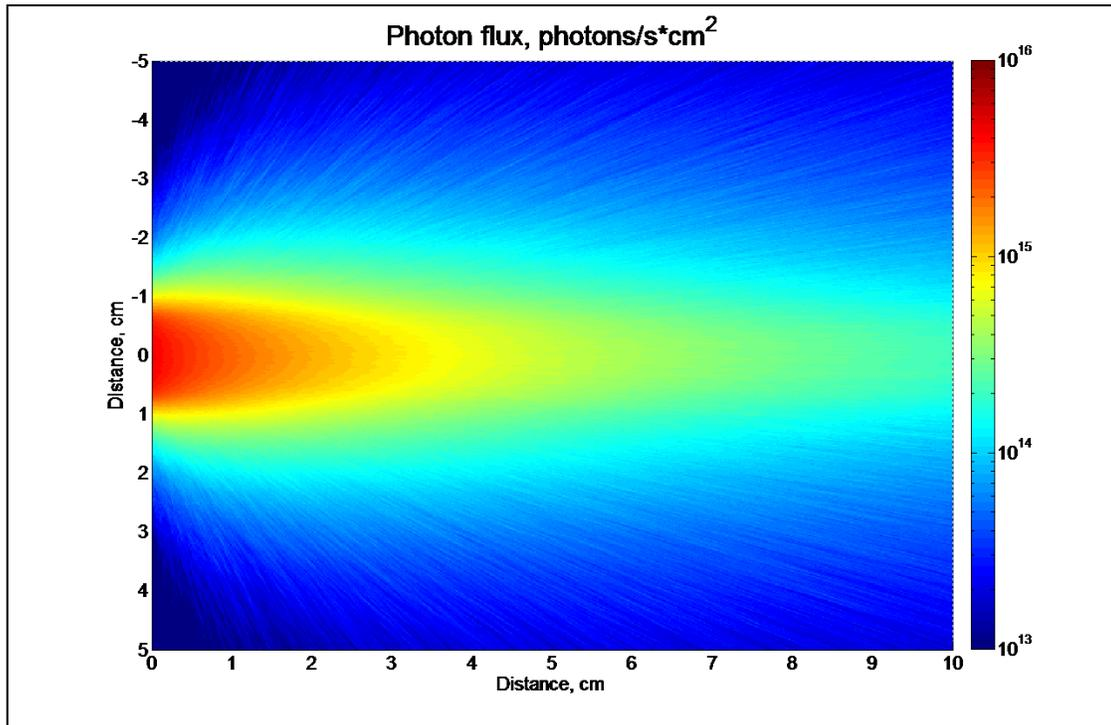
Figure 12. MCNPX simulations results for photon flux generated by a tungsten converter. The 40 MeV electrons are incident from the left. A 10 kW beam is assumed for the simulations.
