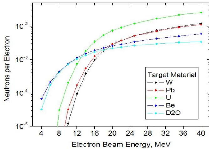
Figure 4. Average neutron flux through a target as a function of the electron beam energy for different target materials.
