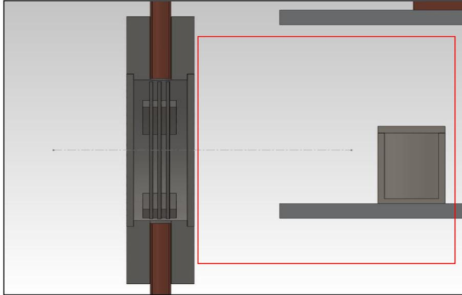
Figure 11. A schematic drawing of the photon source. Water-cooled tungsten converter plates will generate bremsstrahlung photons which will activate sample material. A conveyer belt system will be used for quick multiple sample activation. A right cylinder region (10 cm x 10 cm) shown in red was used for photon flux simulations below (Figure 12).
