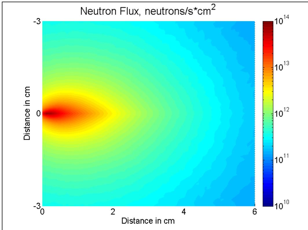
Figure 6. MCNPX simulations results for neutron flux through the tungsten cylinder 6 cm long and 3 cm in radius (shown as black contour line). The 40 MeV electrons are incident from the left. 10 kW beam is assumed for the simulations.
