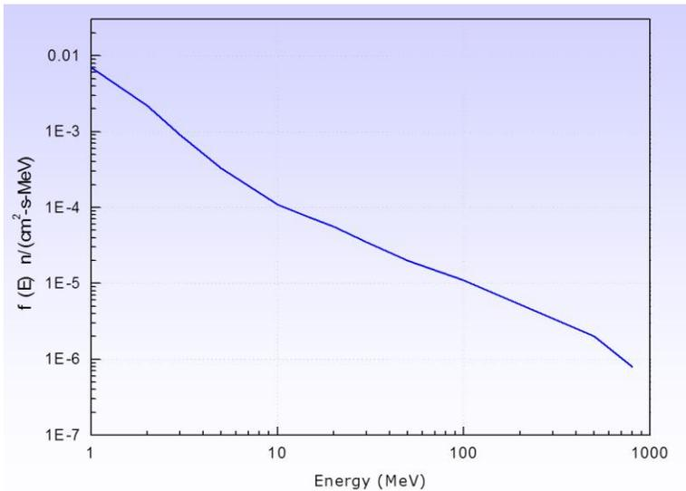
Figure 1. Atmospheric neutron energy spectrum.
