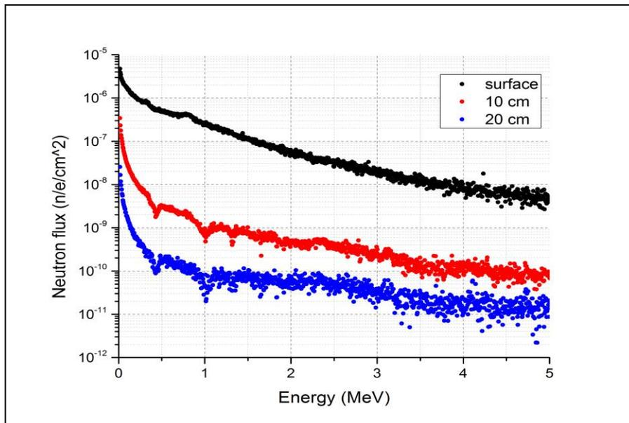
Figure 8. MCNPX simulations results for neutron energy distribution through the tungsten target and D<sub>2</sub>O moderator. Neutron flux is calculated per incident electron!
