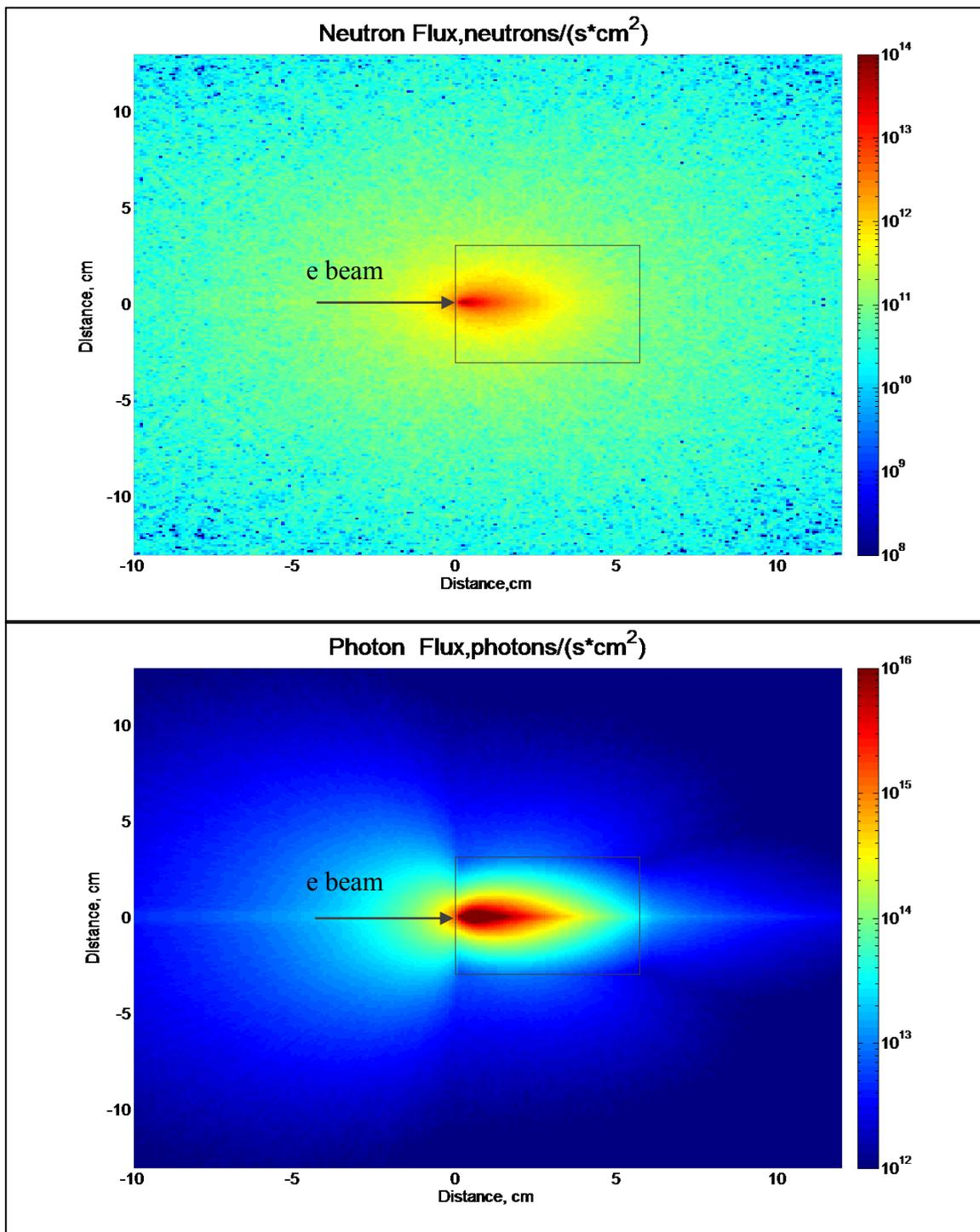
Figure 9. MCNPX simulations results for neutron flux (top) and photon flux (bottom) through the tungsten cylinder surrounded by a thick layer of D<sub>2</sub>O. The 40 MeV electrons are incident from the left. 10 kW beam is assumed for the simulations.
