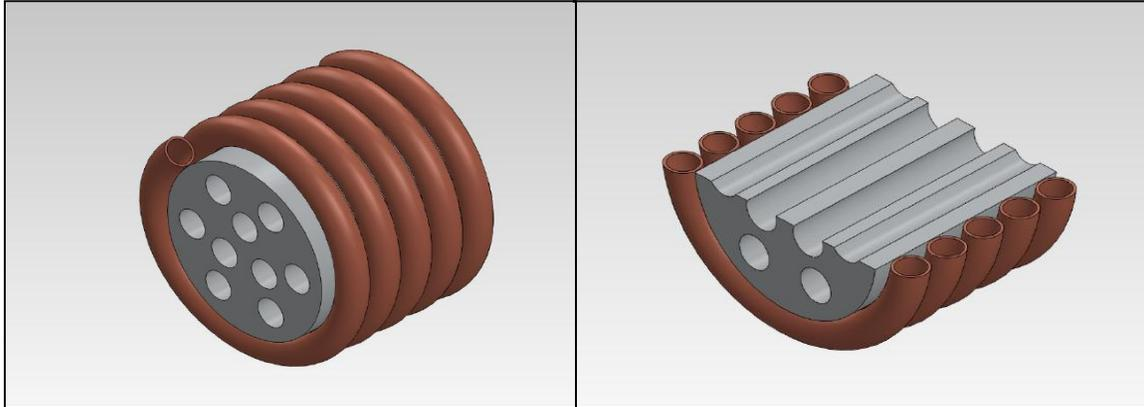
Figure 5. A schematic drawing of the fast neutron source. A high Z material cylinder will have cavities for sample. Water cooling will be enough for 10 kW, for higher powers other cooling schemes need to be designed.
