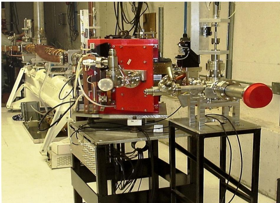
*Figure 3. 10 kW 40 MeV LINAC. The proposed testbed will be placed right at the end of the beamline, surrounded by a thick concrete shielding wall.*
