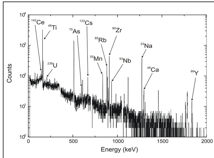
Figure 10. A typical spectrum obtained at the Idaho Accelerator Center by placing an irradiated sample in the high-purity germanium detector. The parent nuclides are labeled with each peak.
