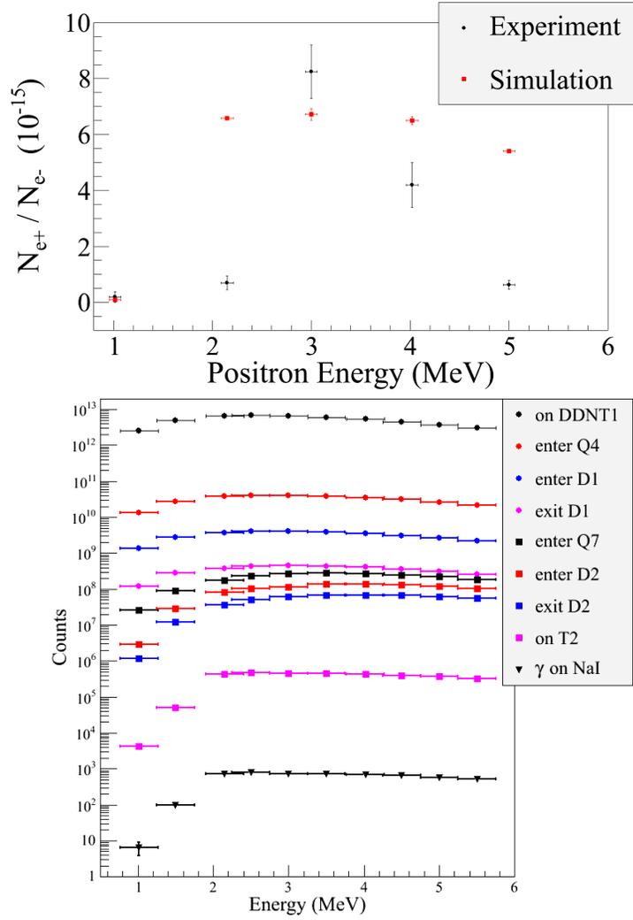
Figure 7: Top: a comparison between the observed positron to electron ratio and a simulation. Bottom: a simulation's beam loss prediction at several locations along the beam line.
