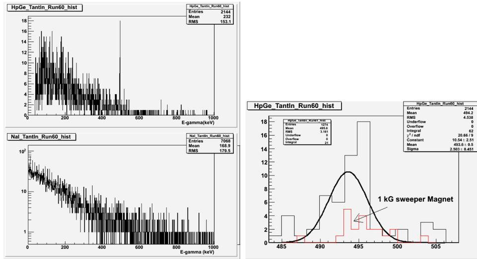
Figure 2: The left figure is the observed photon energy distributions as measured by the HpGe (top) and NaI (bottom) detectors. There was no coincidence requirement using the two detectors. The right figure is the HpGe photon energy distribution before and after a sweep magnet is used to deflect charged particles away from the annihilation target.
