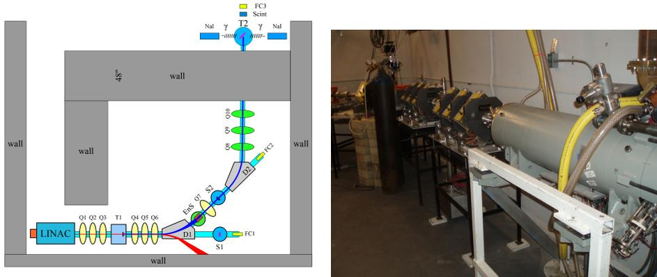
Figure 3: Left: a block diagram describing the new beam line constructed for this project. Right: a picture of the linac and the zero degree line.
