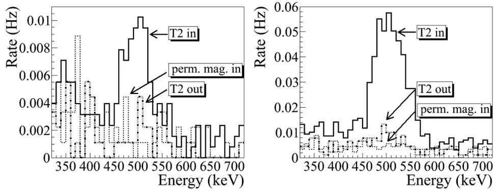
Figure 6: The coincidence signal observed in the beam left and beam right NaI detectors when T2 is in, T2 is in along with a magnet, and when the magnet is removed and T2 is out. The right figure correspond to the beam right detector.
