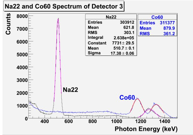
Figure 5: NaI detector calibration using a Na-22 (0.511 & 1.27 MeV lines) and a Co-60 source (1.17 & 1.33 MeV lines).
