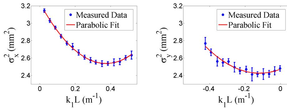
Figure 4: The top figure depicts the OTR apparatus. The bottom left (right) figure represent the measured change in the beam spot size along the vertical (horizontal) direction when the quadrupole field strength changes.
