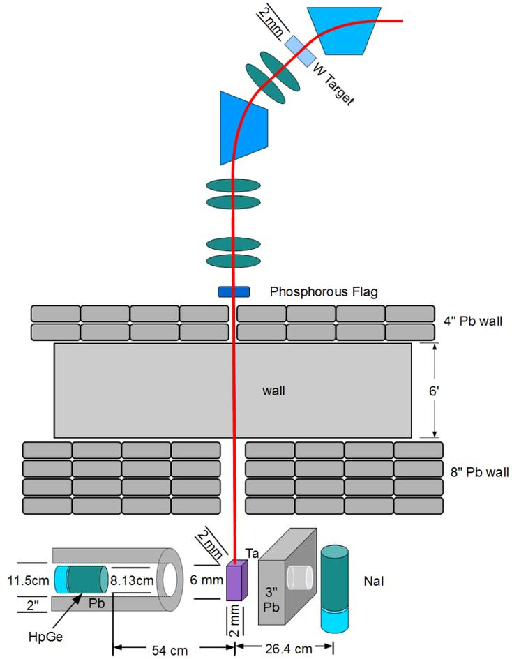
Figure 1: A block diagram of the beam line used for an initial set of positron production measurements
