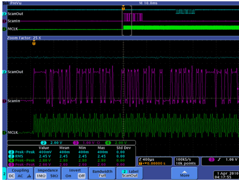
Figure 4-7: Single VFAT ScanIn PBRs with base 8 bit patter
