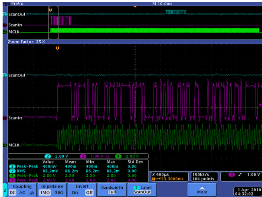
Figure 4-9: Daisy-Chained VFATs ScanIn bit patter
