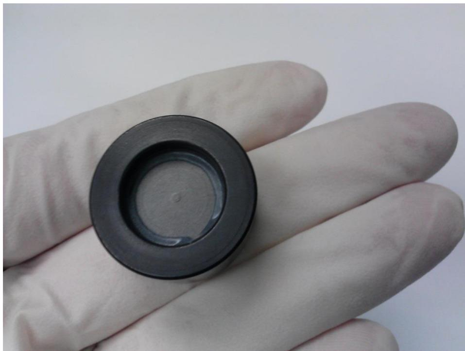
**Figure 5.1:** Sealed sample chamber containing 1.0  $\mu\text{g}$  cesium behind 1.0 mm IG-110 graphite barrier (uncured cement)
