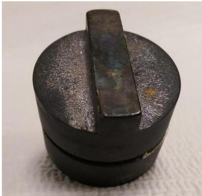
**Figure 9.6:** Molybdenum container after annealing attempt, with dark purple MoO<sub>2</sub> oxidation layer visible
