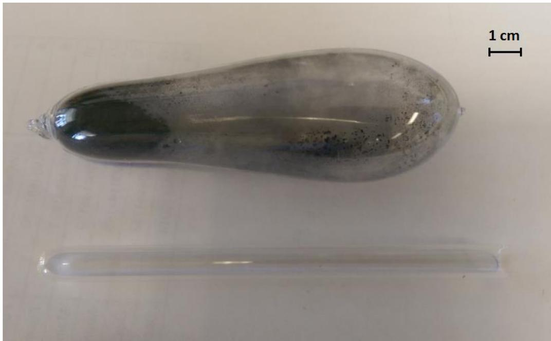
**Figure 9.3:** Sealed quartz tube after annealing procedure
