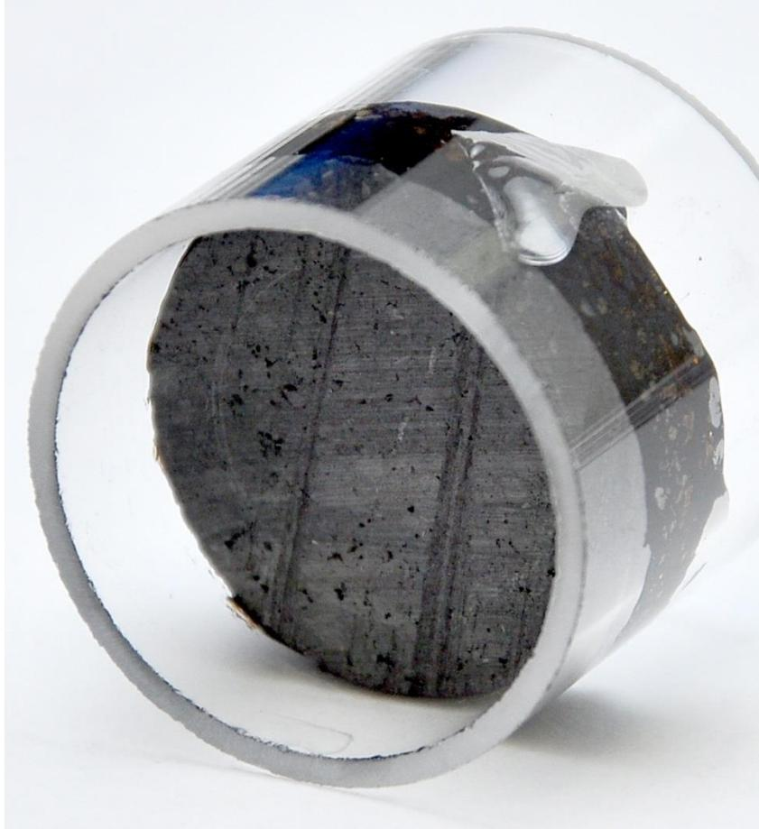
**Figure 4.13:** Graphite disc bonded to quartz tube using Aremco Graphi-bond, after curing procedure. Note cracking in quartz tube at 2 o'clock position and air bubbles distributed around the edges of the barrier.
