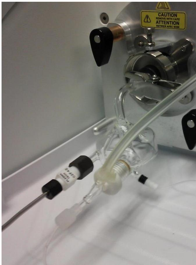
**Figure 6.3:** Dual inlet spray chamber. Inlet 1 (left) from He-jet with He flow rate of 1 L/min. Inlet 2 (right) from nebulizer that injects 200  $\mu\text{L}/\text{min}$  of 1.00 ng/g In as an internal standard.
