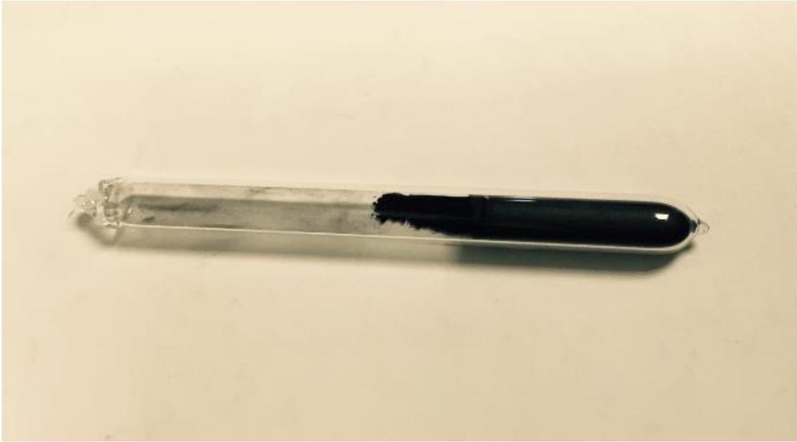
**Figure 9.2:** Sealed quartz tube containing 1 g graphite powder and five R=1/16" IG-110 spheres before annealing procedure
