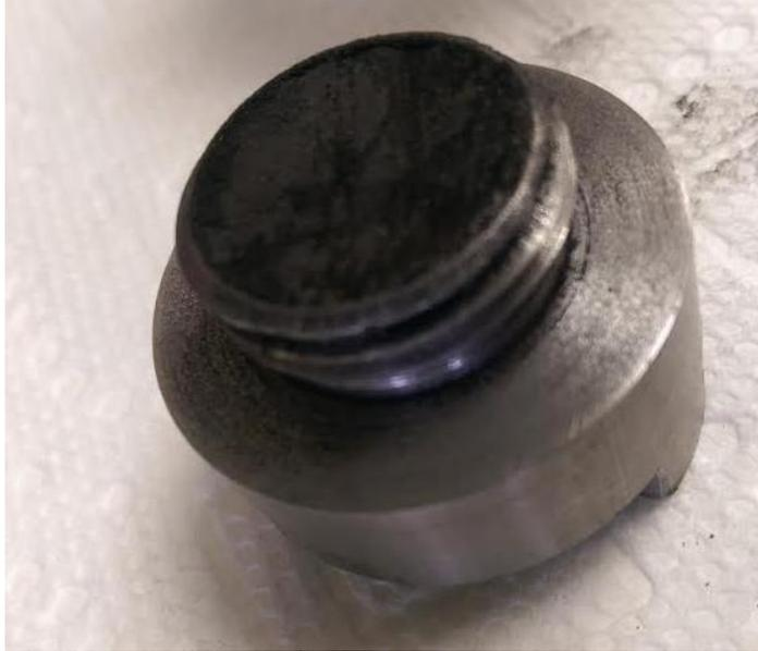
**Figure 9.5:** Molybdenum container filled with Sr laden graphite powder and IG-110 spheres
