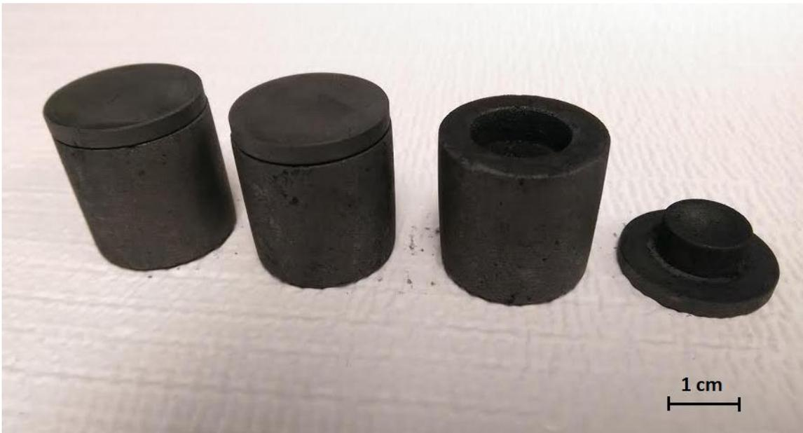
**Figure 9.7:** Annealed graphite canisters
