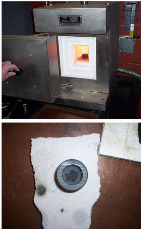
**Figure 4.7:** Aremco 890 SiC-Graphite seal at start (top) and end (bottom) of 900° C, 10 hr heating cycle under argon atmosphere
