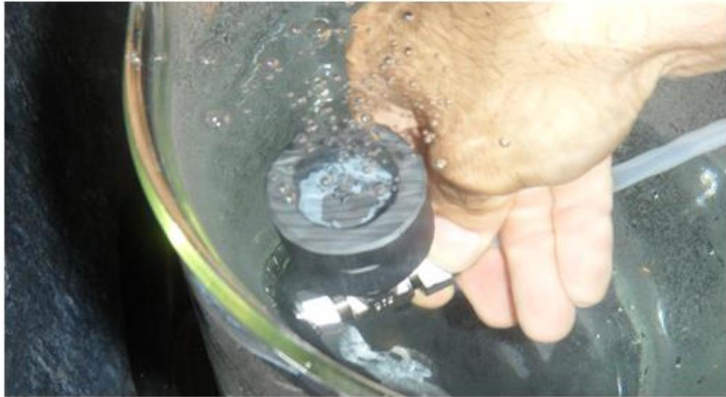
**Figure 4.8:** Aremco 890 graphite-SiC seal during helium permeation experiment.
