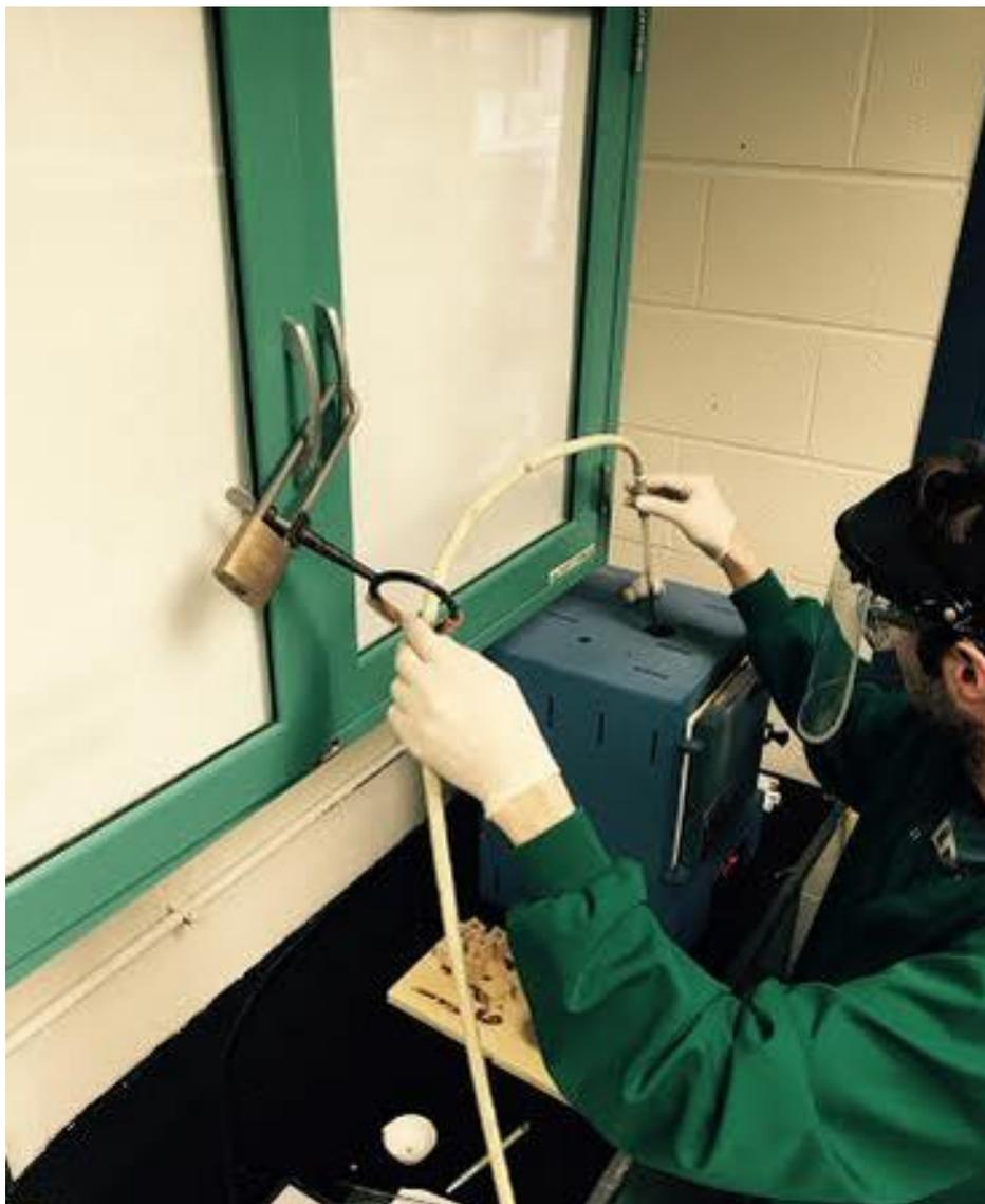
**Figure 9.1:** Metal nitrate decomposition under vacuum in quartz tubing
