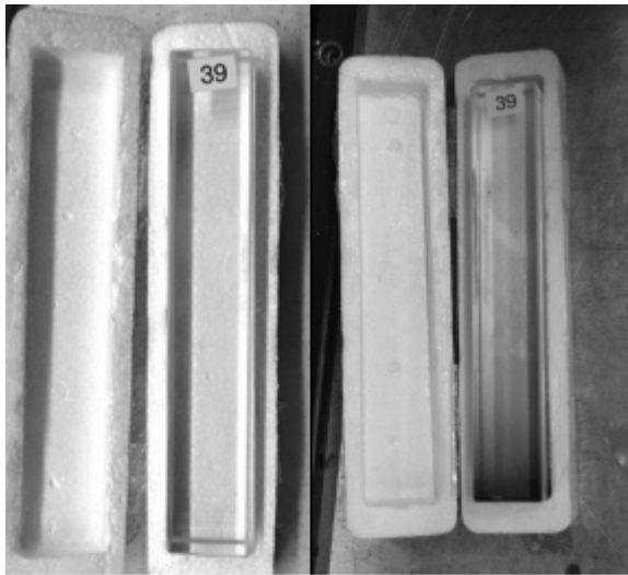
1 2 Figure 5. Photographs of block 39 before (left) and after (right) irradiation.
