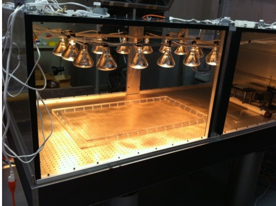
Figure 6: IR array for stretching 100 cm X 50 cm GEM foil for proposed CMS upgrade.
