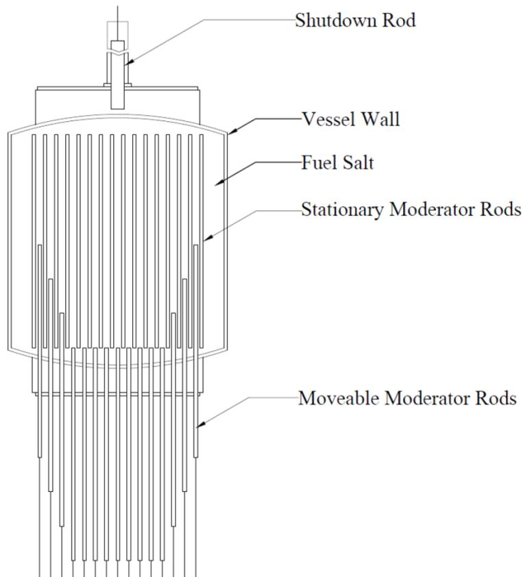
**Figure 2-1 TAP Schematic Showing Moveable Moderator Rods [2-2]**
