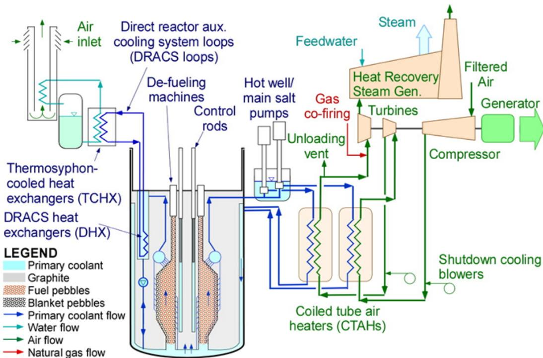
Figure 2-5 Mark 1 PB-FHR Flow Schematic [2-14]
