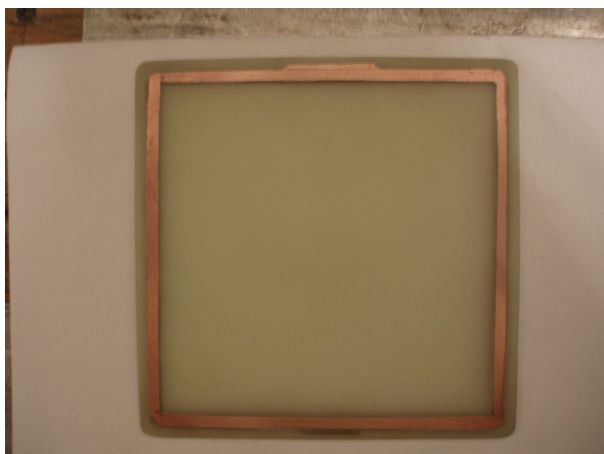
Figure 4: A copper frame on FR4.
