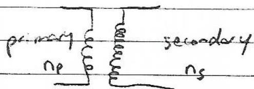
$$\text{Voltage gain} \quad \frac{V_s}{V_p} = \frac{n_s}{n_p}$$
