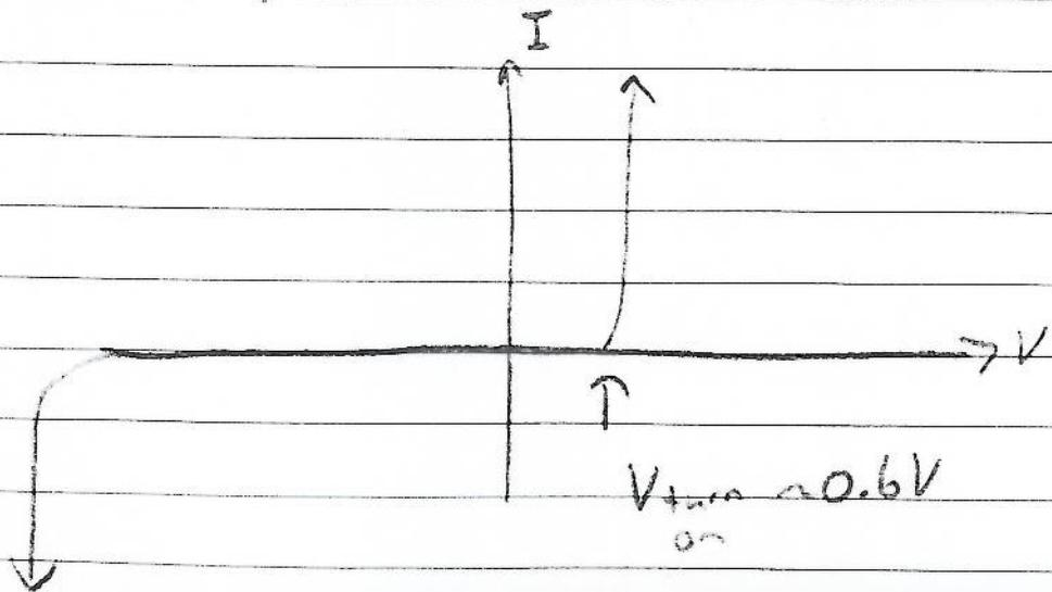
Since B-E junction is forward biased  $V_{BE} \approx 0.6V$  (small)
