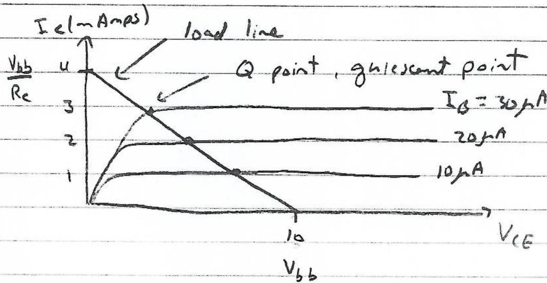
$$I_c = \frac{V_{bb}}{R_c} \quad \text{transistor fully turned on}$$
