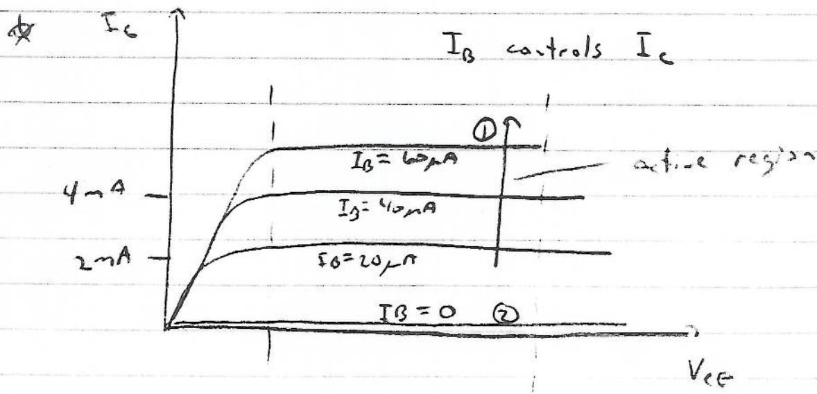
$I_C$  independent of  $V_{CE}$ , but increases as  $I_B$  increases
