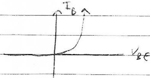
Small  $\Delta V_{EB} \rightarrow$  large  $I_B \rightarrow$  even larger  $I_c$
