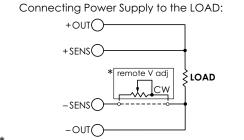
$^st$  THE DOTTED LINE CONNECTION IS REQUIRED, unless remote voltage adjustment is used.
