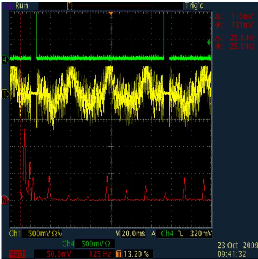
Figure 4 shows a very clear response from the field wire at 25Hz and note that the amplitude of the response has a significant amount of other frequency components.
