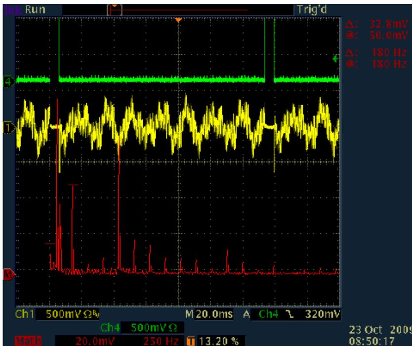
Figure 1 shows the pulse width and repetition of the tension circuit's pulse structure (Green trace)
