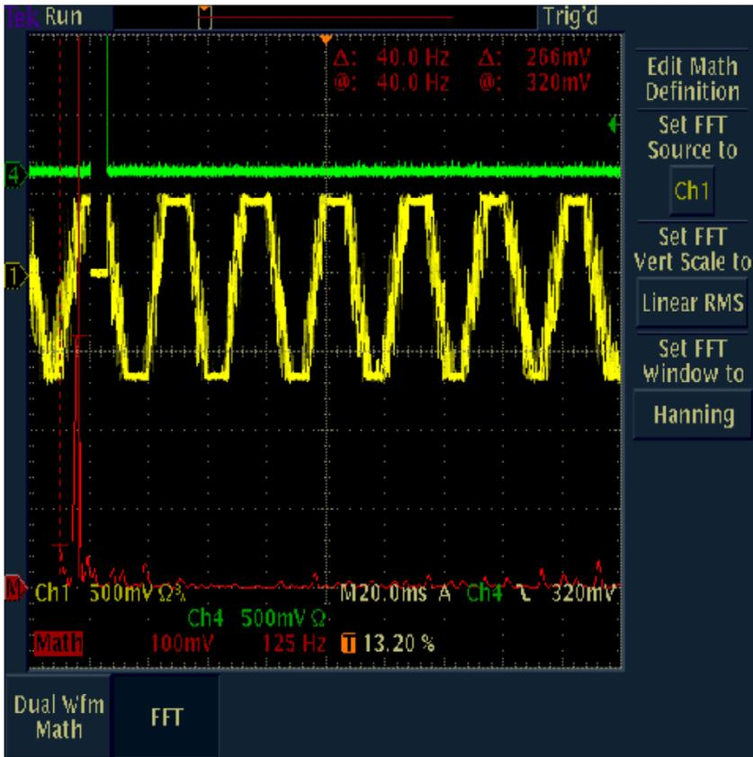
Figure 3 shows a very clear response from the sense wire at 40Hz and note that the amplitude of the response is saturating the amplifier. One could measure the frequency without the FFT match function!
