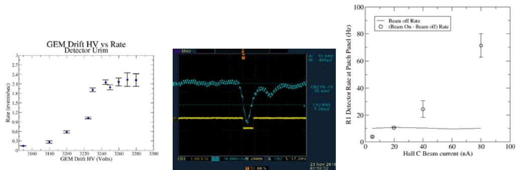
Figure 3. Qweak GEM detector signals. The left most figure shows how the Cosmic rate in the detector approaches the expected 2 Hz rate as a function of GEM Drift/amplifier voltage. The middle picture is the output captured by an oscilloscope. The right most figure illustrates how the detector rate increased with the Hall C beam current.
