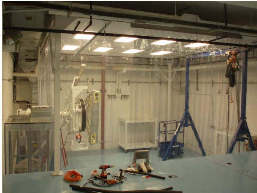
Figure 1. The ISU cleanroom. A R1 drift chamber is shown mounted on the stringing platform. Particle counter measurements show the room is within a class 10,000 rating.
