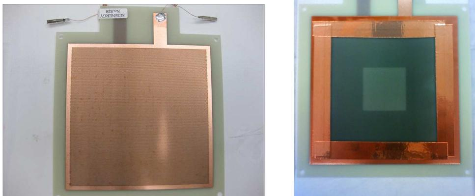
**Figure 1.** The plane view of TGEM (left) and RETGEM (right).
