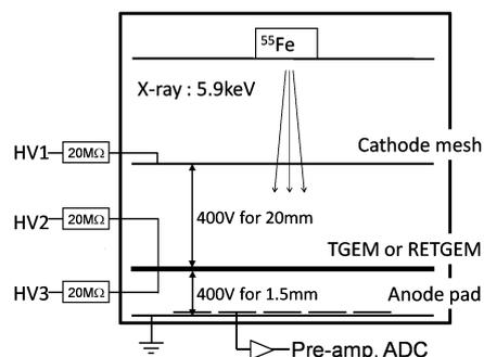
**Figure 3.** The schematic view of test setup
