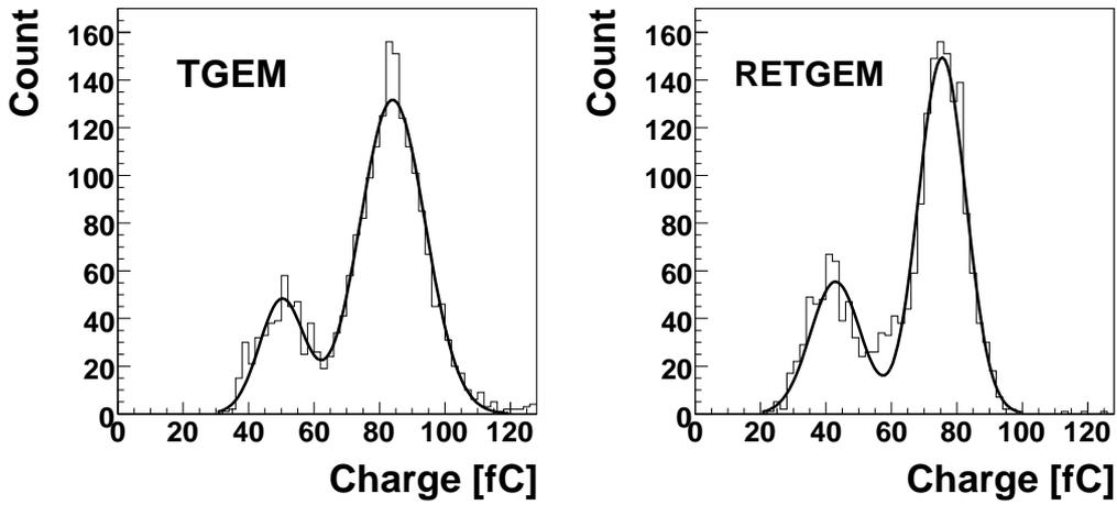
Figure 4. The charge distributions for TGEM and RETGEM.
