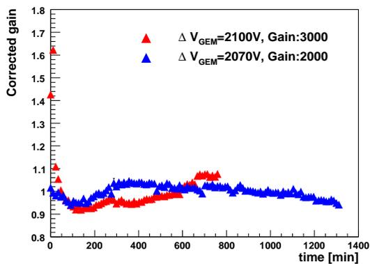
**Figure 7.** The P/T dependence of the relative gain of TGEM.
