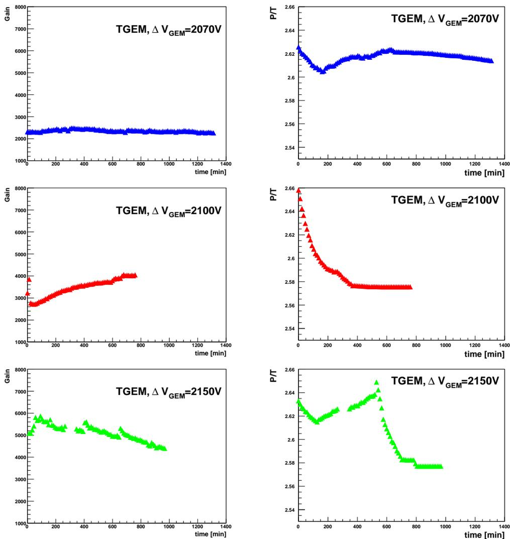
**Figure 6.** Left: Gain variation as a function of TGEM with  $\Delta V_{GEM}=2070$  V, 2100 V and 2150 V. Right: Time variation of P/T during the measurement.
