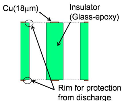
**Figure 2.** The cross sectional figure of TGEM with rim.
