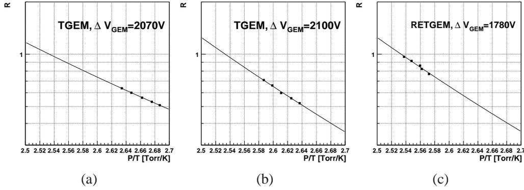
**Figure 8.** Gain dependence of P/T. (a): TGEM with  $\Delta V_{GEM} = 20700$  V. (b): TGEM with  $\Delta V_{GEM} = 2100$  V. (c): RETGEM with  $\Delta V_{GEM} = 1780$  V.
