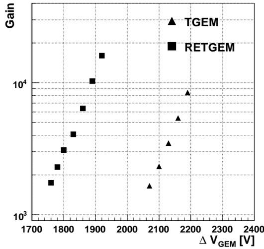
Figure 5. The voltage dependence of gain of TGEM and RETGEM.
