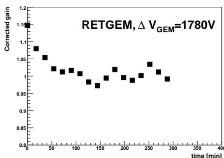
**Figure 10.** The corrected gain of RETGEM. The data are normalized by the mean value of datum.
