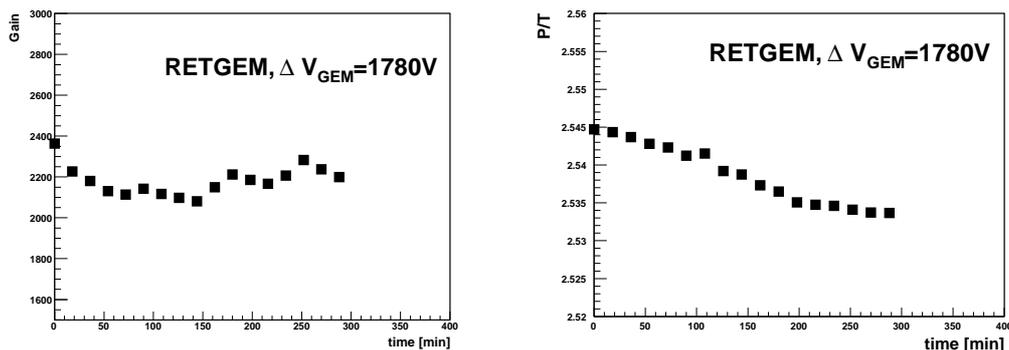
**Figure 9.** Left: Gain variation as a function of time of RETGEM with  $\Delta V_{GEM}=1780$  V. Right: The P/T value during the measurement.
